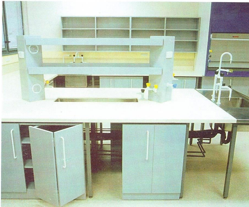
Plate 31 Typical laboratory workbench with movable under-bench storage units (Case study 8) ▼
